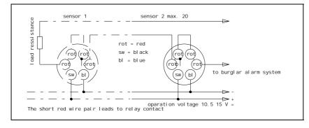
One or up to 20 **GBD** detectors can be wired in series according to the connection diagram including a termination resistor (4.7 – 22K Ohm). The wires of red and white are the relay output wires, the wires of yellow and brown are anti-tamper loop
